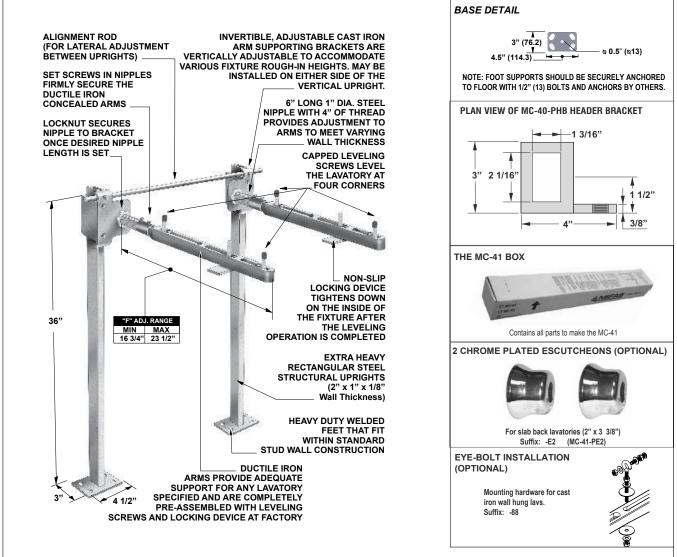
MC-41 Series Meets ANSI/ASME fixture carrier standard A112.6.1M-97 250 Lb. Load Rating NOTE: See the various fixture dimensional rough-in guides on the www.mifab.com website.
