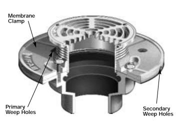
body had to be designed that allowed weepholes to remove water that may seep around the rim of the drain. Since then, architects and mechanical designers have been able to specify products that featured a variety of design considerations that were made necessary by the rapidly changing building techniques we have experienced since the beginning of the twentieth century.
