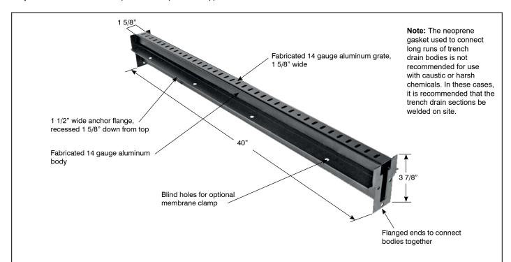
**Note:** Specify the total length of the T5000-158 trench drain system required along with the type of grates required, number of outlets (specify bottom or end or both) and design of the trench drain system (straight run only or straight runs with corners and turns).
