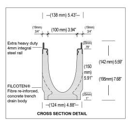
**Load Class Definition:** Load Class C - Heavy Duty, DIN 19580, 56,000 lbs. 1,162 psi. For commercial pneumatic tire traffic patterns and tractor trailers.
