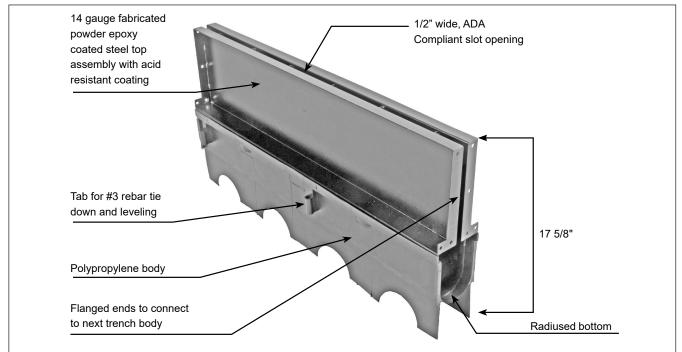
**Note:** Specify the total length of the T1400-SD-18H slot drain system required along with the number of outlets (specify bottom or end or both) and design of the trench drain system (straight run only or straight runs with corners and turns).
