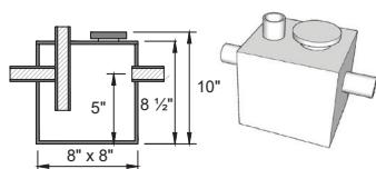
SEALED RECTANGULAR TANK WITH TOP OR SIDE INLET, OUTLET, AND CLEANOUT.
