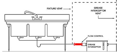
C. Without external flow control, directly connected "Internal flow control". Recognized per ASME/CSA
