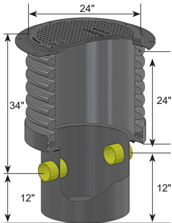
HDPE body with 4" no hub inlet and outlet with offset fall for accurate sample results. Below ground installation with 24" diameter double wall corrugated pipe (supplied by others). H-20 load rated ductile iron, gasketed and bolted, pickable 27" diameter cover.
