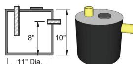
ROUND TANK WITH FEMALE TOP INLET, SIDE OUTLET, WELDED OVER, AND THREADED CLEANOUT.
