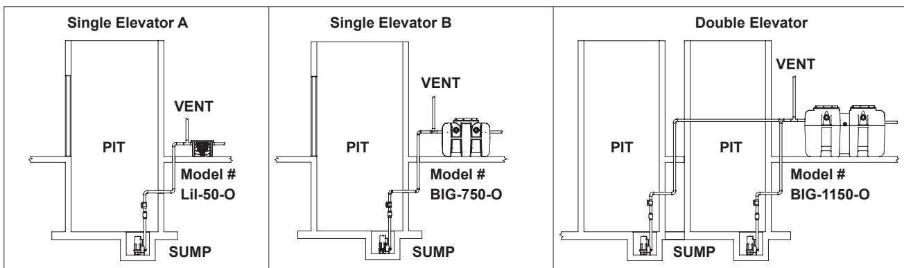
Note: The MIFAB® coalescing pack should be specified with all oil interceptors receiving pump fed oil waste water because the emulsification of the oil from the pump.
