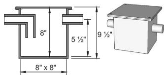
SIDE INLET AND OUTLET WITH BOLTED AND GASKETED COVER.
