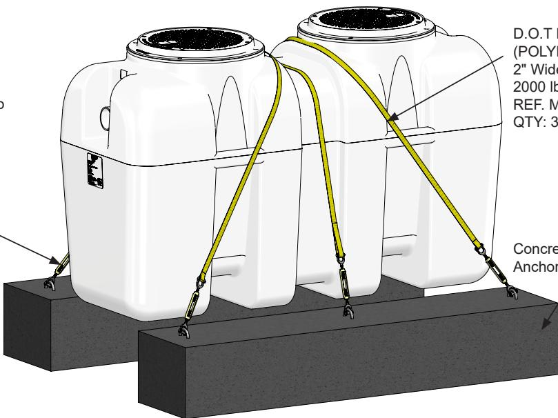
The BIG-1150-AK-SET-2 is used when greater hold down strength is required. The polyester tie-down straps and turnbuckles are rated at 2,200 lbs. working load each.
