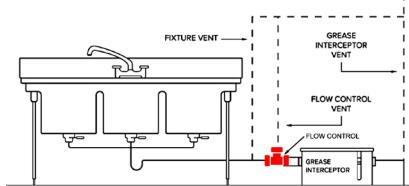
B. External flow control without air intake, directly connected. Recognized per ASME/CSA
