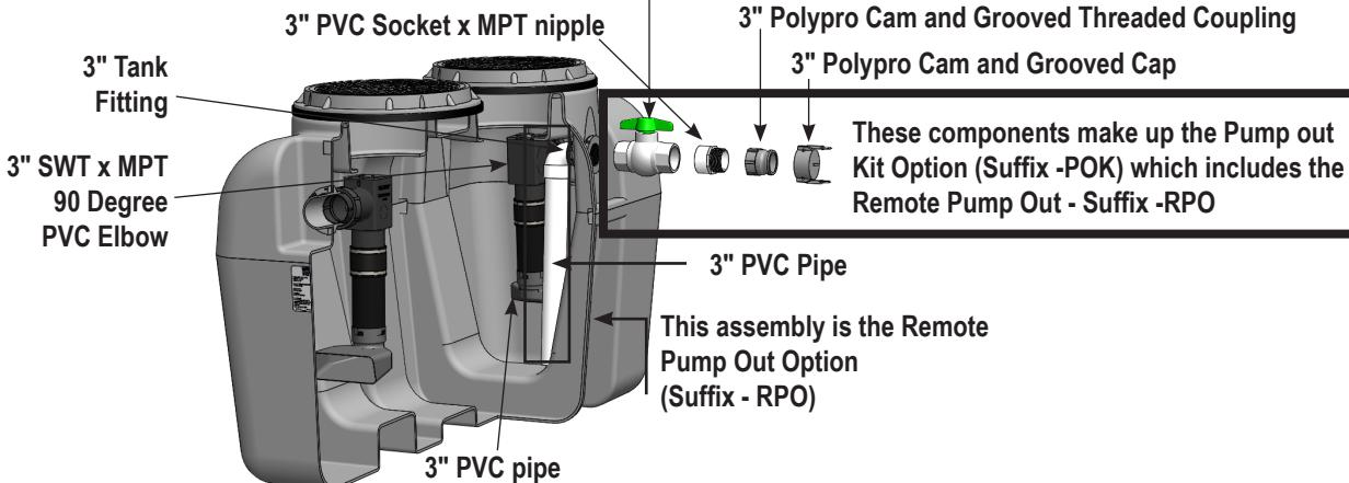
These components make up the Pump out Kit Option (Suffix -POK) which includes the Remote Pump Out - Suffix -RPO
