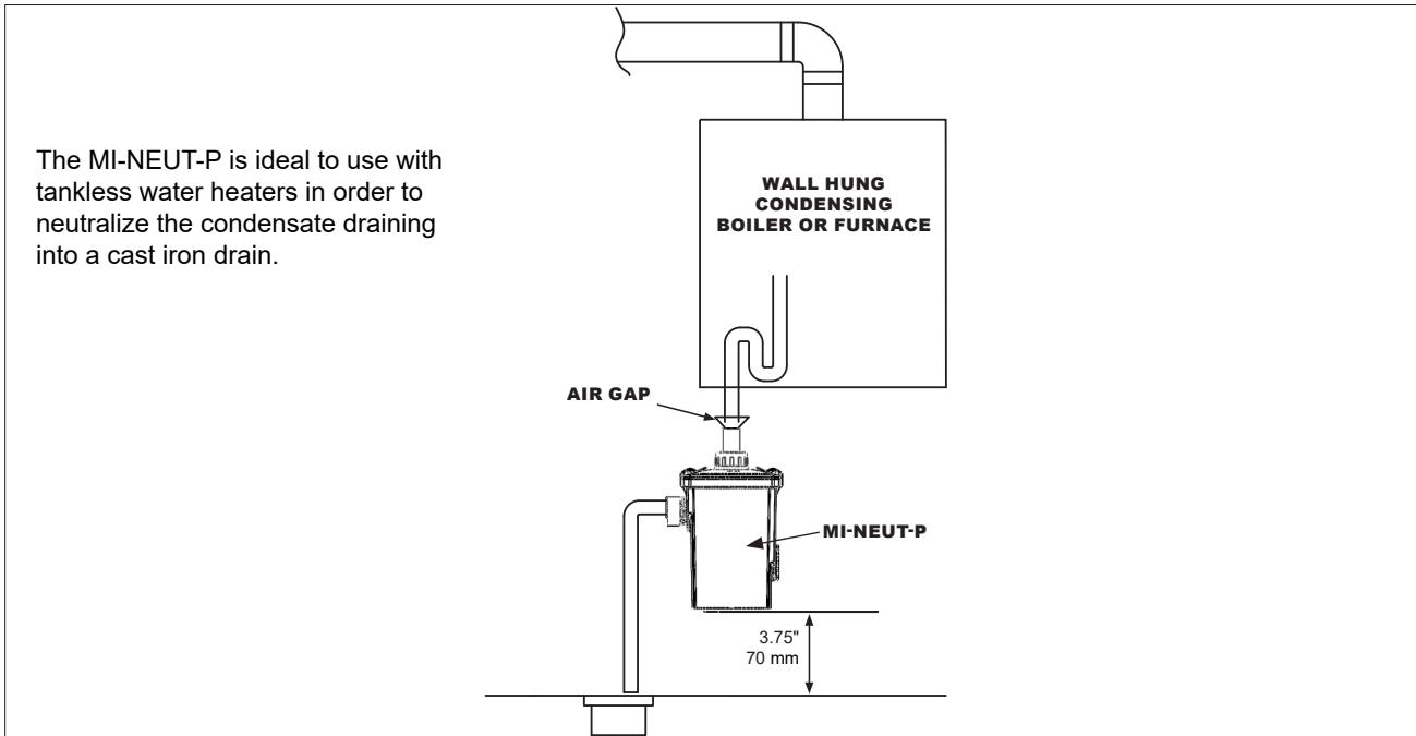
The MI-NEUT-P is ideal to use with tankless water heaters in order to neutralize the condensate draining into a cast iron drain.
