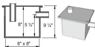
TOP INLET AND SIDE OUTLET WITH BOLTED AND GASKETED COVER.
