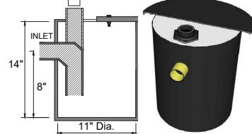
TOP INLET. IT HAS A HALF-WELDED COVER WITH FEMALE THREADED TOP INLET, SIDE OUTLET, &amp; HALF COVER FOR SERVICING.
