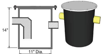
STANDARD 5 GALLON POINT OF USE TANK. IT COMES WITH 1 1/2" OR 2" FITTINGS &amp; BOLTED COVER.
