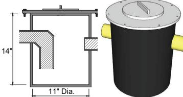
ADDITION OF AN 8" THREADED MANWAY IN THE COVER FOR EASY SERVICING.
