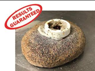
Mini Max® filter filled with solid waste
