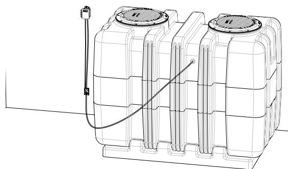
**HIGH LEVEL ALARM:** MIFAB® offers 2 High Level Alarm options; a single float and dual float option. The purpose of the High Level Alarm is to monitor and send an audible and visual alarm when the interceptor's grease or oil capacity is approximately 75% full. (Specify suffix -HLA) High level alarm systems can be installed on any MIFAB® grease or oil interceptors to allow the owner to monitor grease and oil levels. This permits the interceptor to be maintained when required.
