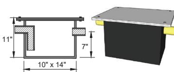
5 GALLON UNDER SINK NEUTRALIZATION TANK WITH 1 1/2" OR 2" FITTINGS AND BOLTED COVER.
