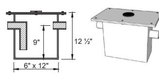
SIDE INLET AND OUTLET WITH THREADED CLEANOUT.
