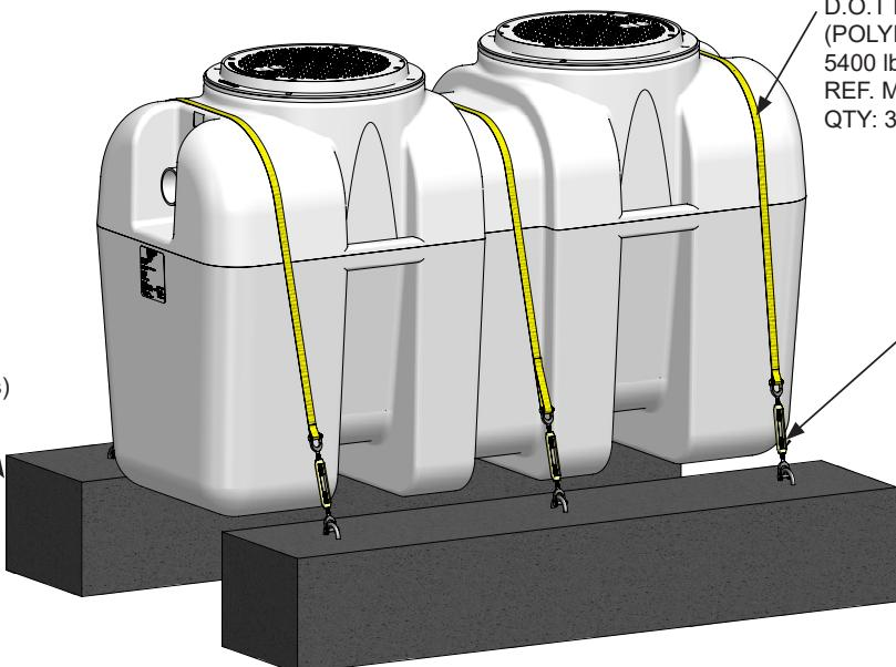
The BIG-1150-AK-SET-3 is used when greater hold down strength is required. The polyester tie-down straps are rated at 4,000 lbs. working load each and the turnbuckles are rated at 5,200 lbs. each.
