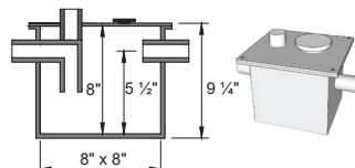
HAS A CLEANOUT AND IS AVAILABLE WITH A TOP OR SIDE INLET AND SIDE OUTLET.
