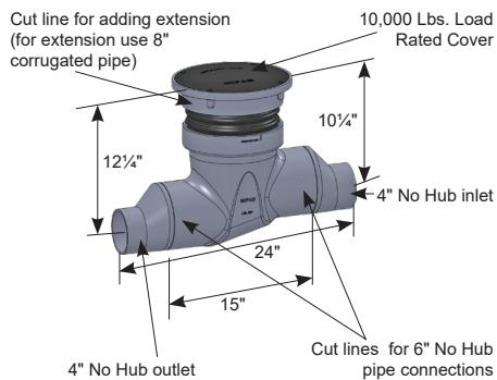
Compact HDPE assembly with 4" no hub inlet and outlet with offset fall for accurate sample results. Sloped body design to reduce solid and grease buildup. Cut lines on body for 6" no hub inlet and outlet. Above ground installation and cut line on body for below ground extension using 8" diameter double wall corrugated pipe (supplied by others). 10,000 lb. load rated HDPE gasketed and bolted 10" diameter cover.
