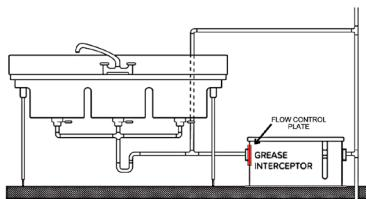
D. Without external flow control, indirectly connected "No flow control". Recognized per ASME/CSA
