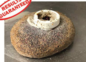
Mini Max® filter filled with solid waste
