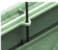
STEP 5 Tighten the zip ties around the pins of the interceptor or through outside of extension and rim of Lil the next hole if using more than one extension.
