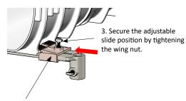
2. Push the adjustable slide against the channel lower profile until tight engagement.
