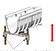
4. Adjust to desired height, secure the installation device by tightening the two wing nuts.
