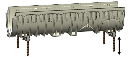
5. ALIGN THE MALE SIDE OF THE NEXT CHANNEL TO THE CONNECTOR; CHANNEL NARROW EDGE SHALL REST INTO DESIGNATED CONNECTOR GROOVE.
