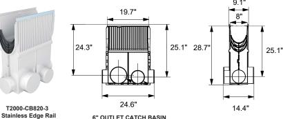
6" OUTLET CATCH BASIN (8" OUTLET ALSO AVAILABLE) Sediment bucket, 4 filler plates and end cap included
