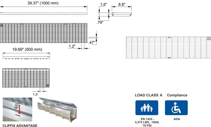
The MEA polymer concrete and GRP channels are designed for our universal CLIPFIX grate locking mechanism. The system (channel and grate) provides longitudinal shift protection.
