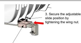
2. Push the adjustable slide against the channel lower profile until tight engagement.
