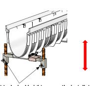
4. Adjust to desired height, secure the installation device by tightening the two wing nuts.
