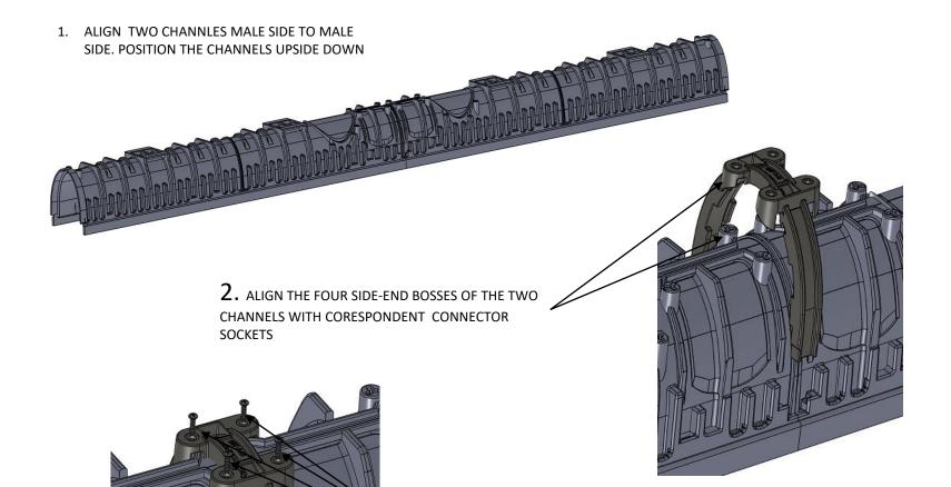
$\begin{array}{l} \textbf{3.} \text{ nest the channels male side bosses into} \\ \text{connector sokets and secure the assembly by} \\ \text{tighten the four provided screws} \ . \end{array}$
