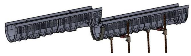
6. MAKE SURE TO ALIGN THE CHANNEL END BOSSES TO CONNECTOR CORESPONDEDNT SOCKETS AND PUSH THE FOLLOWING CHANNEL DOWNWARDS UNTIL COMPLETELY NESTED INTO THE CONNETOR GROOVE; TOPRAILS OF THE CHANNELS SHALL BE ALIGNED AND FLASH WITH EACHOTHER.
