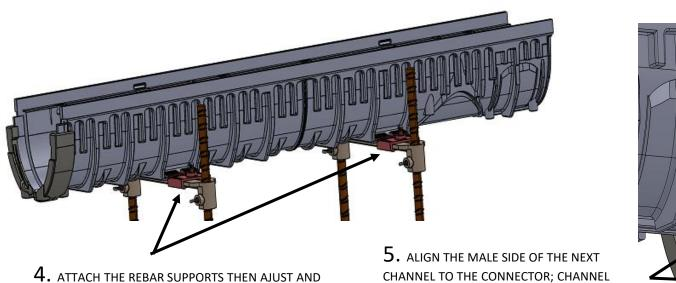
SECURE THE CHANNEL TO RECOMMANDED LEVEL
