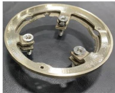
**3** Separate the Shank Ring from the Collar of RTS5-1. Alternatively unscrew the three set screws, few turns at time.
