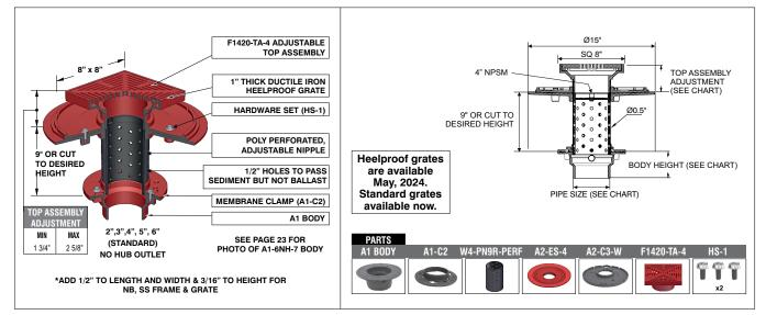
Note: When used as a floor or area drain in exterior areas and subject to rainfall, ensure that the free area is equal to twice the transverse (cross sectional) area of the connecting pipe.
