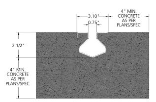
Specifying engineer is responsible for concrete encasement and reinforcing based upon application and local codes.
