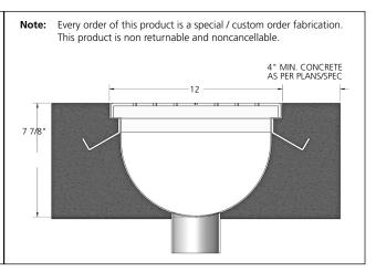
The P4120-LCB is NSF certified with a load classification of Medium Duty.
