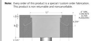
Specifying engineer is responsible for concrete encasement and reinforcing based upon application and local codes.
