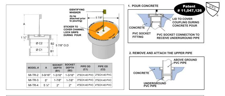
The MI-TR can also be used to receive a medium sweep street 90 fitting from the horizontal waste line from an off the floor water closet carrier fitting. The MI-TR will be installed in the ground, flush to grade, over PVC drain pipe. This allows one or two more water closet carriers to be installed and still have enough vertical space to connect the horizontal carrier fitting waste line with a medium sweep street 90 fitting to the MI-TR transition coupling.
