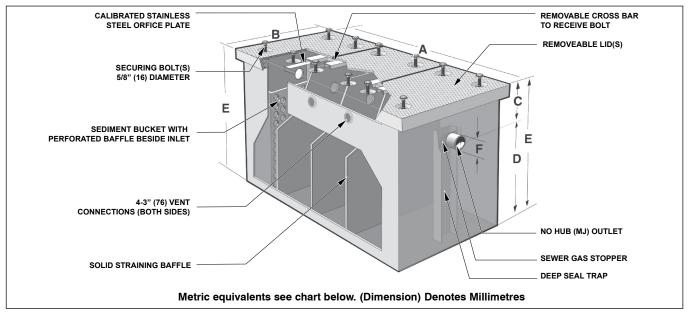
**Note:** The "C" dimension detailed above is from either the middle of the inlet or the outlet to the top the interceptor. The inlet and outlet dimensions are always the same.
