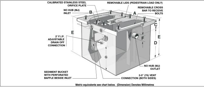
Note: The "C" dimension detailed above is from either the middle of the inlet or the outlet to the top the interceptor. The inlet and outlet dimensions are always the same.
