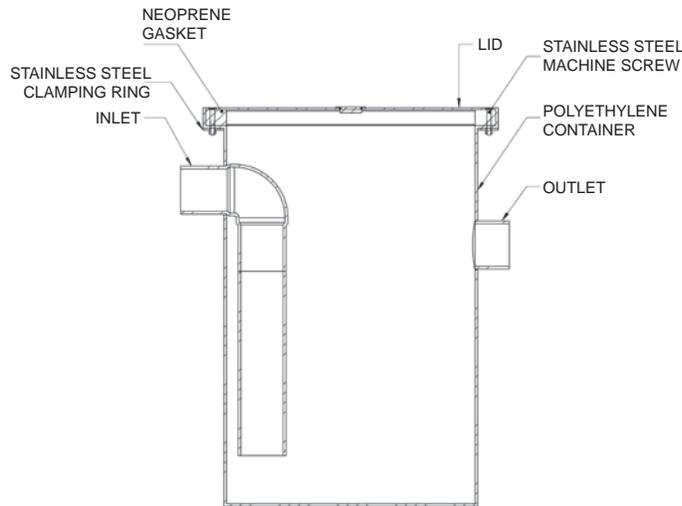
**Sizing:** Local and National Plumbing Codes have different ways of sizing acid neutralization tanks. It is recommended to consult with the Code Officials in your area for their sizing requirements. The most common sizing method is to calculate the number of laboratory sinks draining into the acid neutralization tank and then choosing a corresponding acid neutralization tank to handle the flow from these sinks. (see Sizing Table below)
