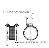
Sizes 2" through 4" Tighten bands alternately to recommended torque.
