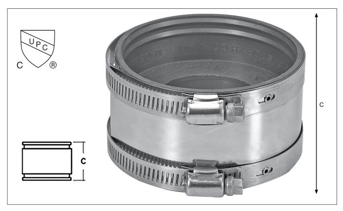
Note: Tighten bolts to 60 inch lbs. min. / max torque. Tested to maintain 4.3 p.s.i. maximum line pressure (10' head pressure) 5/16" driver required to tighten bolts.
