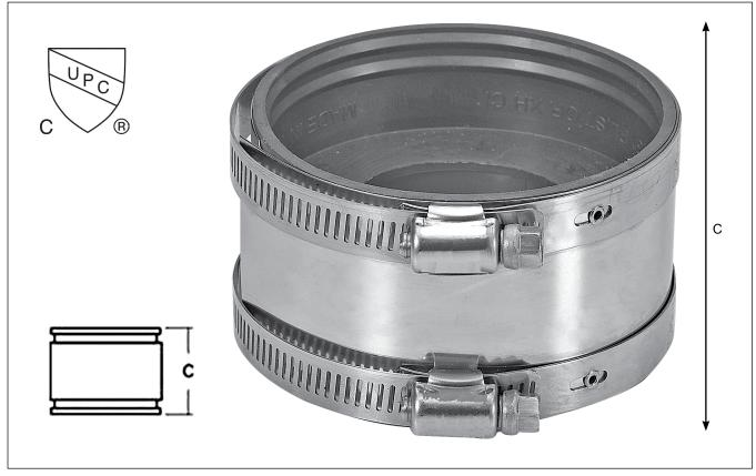
Note: Tighten bolts to 60 inch lbs. min. / max torque. Tested to maintain 4.3 p.s.i. maximum line pressure (10' head pressure). 5/16" driver required to tighten bolts.
