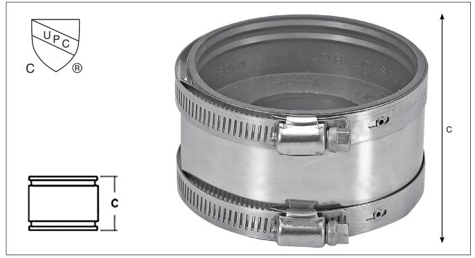
Note: Tighten bolts to 60 inch lbs. min. / max torque. Tested to maintain 4.3 p.s.i. maximum line pressure (10' head pressure). 5/16" driver required to tighten bolts.
