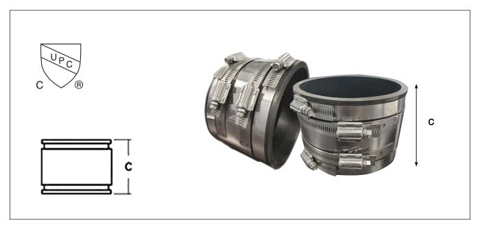
Note: Tighten bolts to 60 inch lbs. min. / max torque. Tested to maintain 4.3 p.s.i. maximum line pressure (10' head pressure) 5/16" driver required to tighten bolts.
