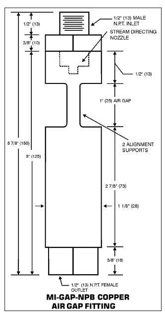
**Application:** MIFAB's MI-GAP-NPB air gap fitting can be used with MIFAB's MR-500-NPB, M1-500-NPB, M2-500-NPB, MI-TSP-1-NPB, MI-TSP-2-NPB, MI-TSP-3-NPB trap seal primers, and MIFAB's MI-DU distribution unit.
