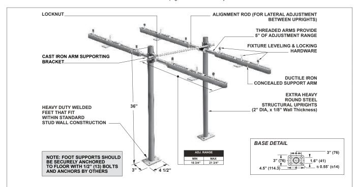
MC-42D-R Series Meets ANSI/ASME fixture carrier standard A112.6.1M-97
