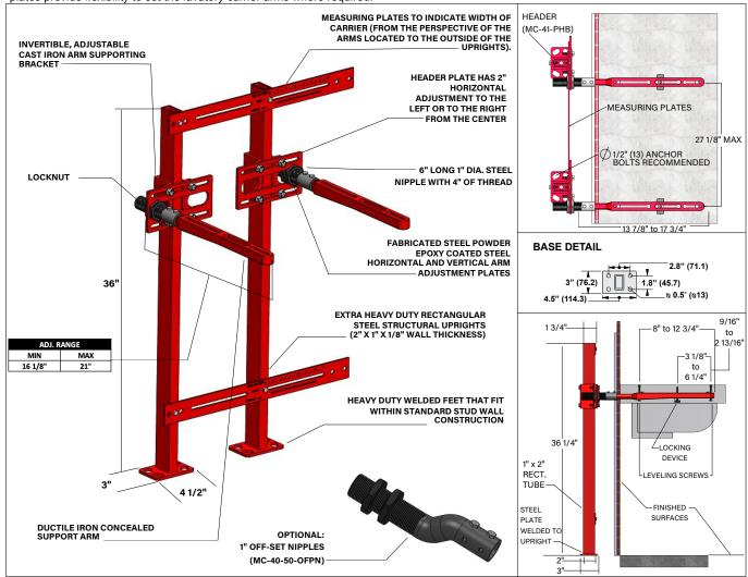
NOTE: FOOT SUPPORTS SHOULD BE SECURELY ANCHORED TO FLOOR WITH 1/2" (13) BOLTS AND ANCHORS BY OTHERS Note: See the various fixture dimensional rough-in guides on the www.mifab.com website.
