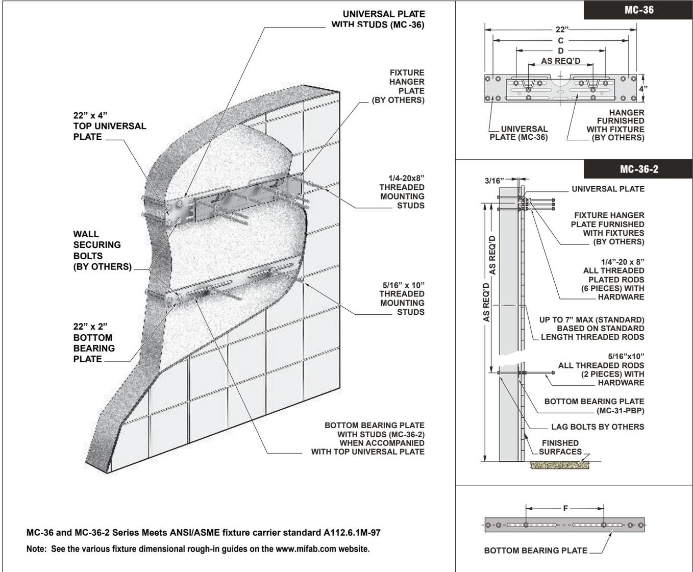
MC-36 and MC-36-2 Series Meets ANSI/ASME fixture carrier standard A112.6.1M-97
