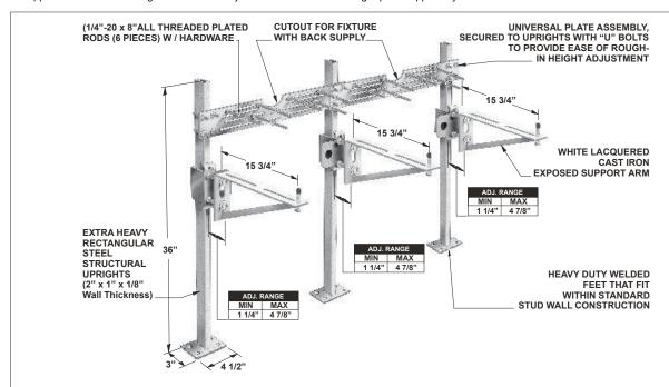
MC-35 Series Meets ANSI/ASME fixture carrier standard A112.6.1M-97
