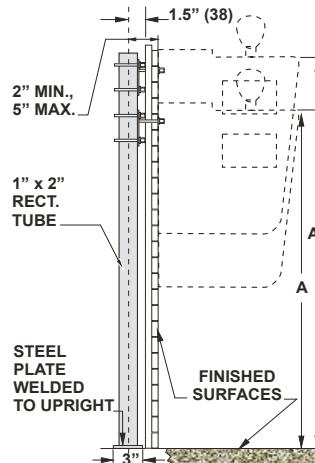
**MC-33 Series Meets ANSI/ASME fixture carrier standard A112.6.1M-97
