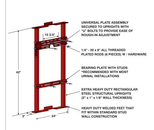
NOTE: Foot supports should be securely anchored to floor with 1/2" bolts and anchors by others
