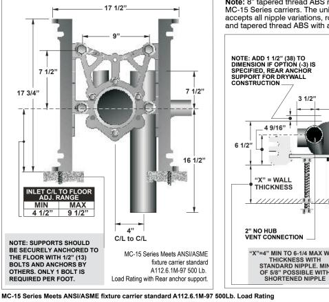
**Note:** 8" tapered thread ABS nipple shipped standard with MC-15 Series carriers. The universal faceplate assembly accepts all nipple variations, rolling thread (-OR), cast iron (-CI) and tapered thread ABS with adjustable horn (-AH).
