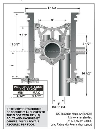
**Note:** 8" tapered thread ABS nipple shipped standard with MC-15 Series carriers. The universal faceplate assembly accepts all nipple variations, rolling thread (-OR), cast iron (-CI) and tapered thread ABS with adjustable horn (-AH).
