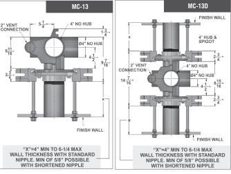
MC-13D Series Meets ANSI/ASME fixture carrier standard A112.6.1M-97 500Lb. Load Rating
