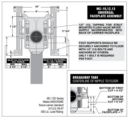
Note: 8" tapered thread ABS nipple shipped standard with MC-13 Series carriers. The universal faceplate assembly accepts all nipple variations, rolling thread (-OR), cast iron (-CI) and tapered thread ABS with adjustable horn (-AH).
