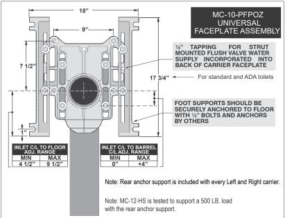
**Note:** 8" tapered thread ABS nipple shipped tandard with MC-10 Series carriers. The universal faceplate assembly accepts all nipple variations, rolling thread (-OR), cast iron (-CI) and tapered thread ABS with adjustable horn (-AH).
