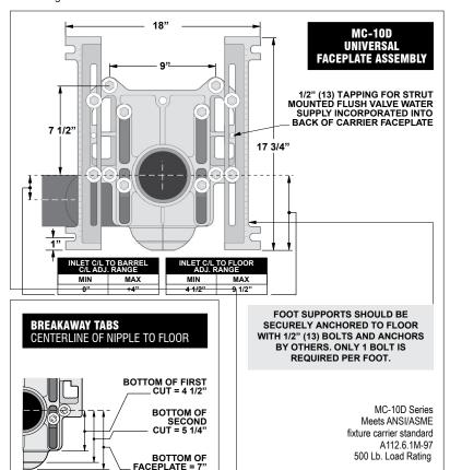
Note: 8" tapered thread ABS nipple shipped standard with MC-10 Series carriers. The universal faceplate assembly accepts all nipple variations, rolling thread (-OR), cast iron (-CI) and tapered thread ABS with adjustable horn (-AH).
