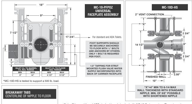
**Note:** 8" tapered thread ABS nipple shipped standard with MC-10 Series carriers. The universal faceplate assembly accepts all nipple variations, rolling thread (-OR), cast iron (-CI) and tapered thread ABS with adjustable horn (-AH).
