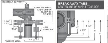
**Note:** 8" tapered thread ABS nipple shipped standard with MC-10 Series carriers. The universal faceplate assembly accepts all nipple variations, rolling thread (-OR), cast iron (-CI) and tapered thread ABS with adjustable horn (-AH).
