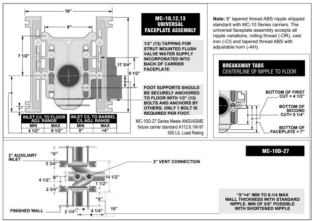
**Note:** 14 1/2" (368) minimum space required between front of foot supports. 9" (229) minimum in wall space required between back of in wall foot supports. **Note:** Foot supports and faceplate are assembled at the factory before shipment in the typical siphon jet water closet configuration and are reversible for the blowout water closet design.
