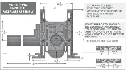
\*MC-10-27-37 is tested to support a 500 lb. load with the rear anchor support.
