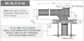
4 1/8" DIMENSION BETWEEN AUXILIARY INLET AND VENT IS IDEAL FOR A STANDARD WYE AND 1/8th BEND CONNECTION
