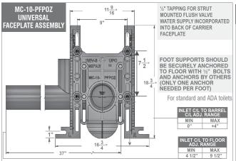
\*MC-10-27-37-HS is tested to support a 500 lb. load with the rear anchor support
