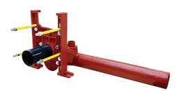
Check out the MC-10-27-37 long barrel carrier from MIFAB. It is standard at 37" long (to allow for the 1" thick partitions between the toilets and is also standard with the -27 auxiliary inlet connection to receive lavatory or urinal waste.
