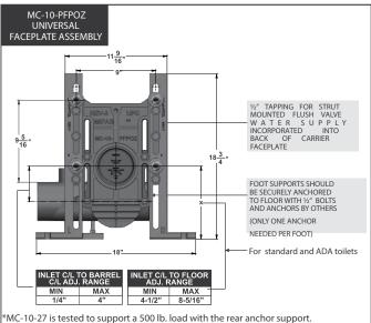
FINISH WALL MC-10R-27 2" NO HUB VENT CONNECTION LOCATED IN LINE WITH NIPPLE. EASY TO CONNECT A WASTE LINE FROM OPPOSITE ROOM 1/2"THREADED MOUNTING POINT "X"=4" MIN TO 6-1/4 MAX WALL THICKNESS WITH STANDARD NIPPLE. MIN OF 5/8" POSSIBLE WITH SHORTENED NIPPLE (SUPPORT STRUT AND CUSHION CLAMP BY OTHERS) FINISH WALL Note: left hand versionsillustrated, right hand are mirror image.
