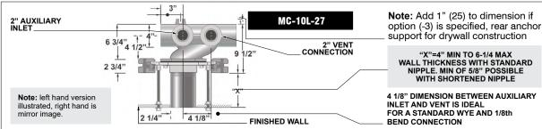
Note: 10 1/2" (267) minimum space required between front of foot and rear of anchor support. 8" (203) minimum in wall space required between back of rear anchor support and back of in wall foot supports.
