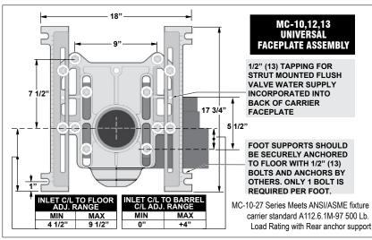
Note: 8" tapered thread ABS nipple shipped standard with MC-10 Series carriers. The universal faceplate assembly accepts all nipple variations, rolling thread (-OR), cast iron (-CI) and tapered thread ABS with adjustable horn (-AH).
